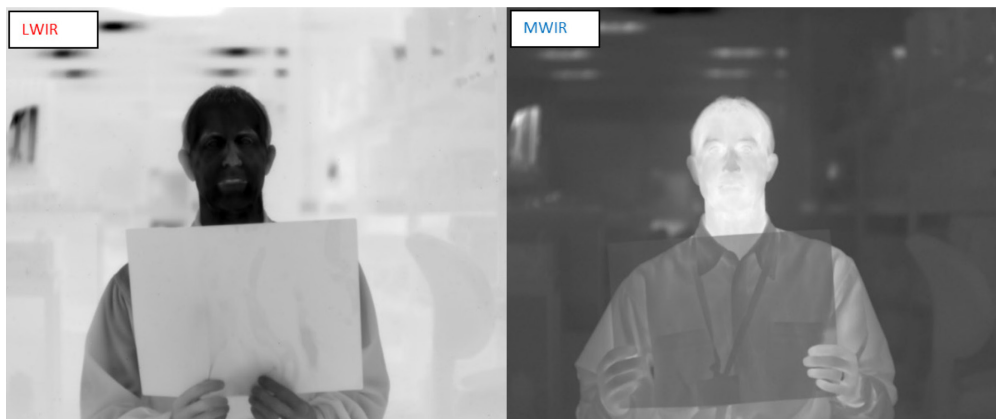
Figure 6: Sample imagery taken from a 12µm pitch, 1280 x 1024 pixel MWIR/LWIR DWB Demo Camera.
